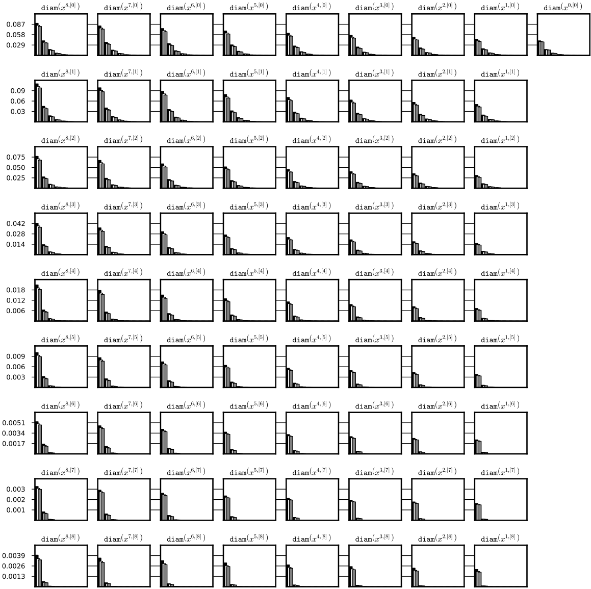
Figure 4.7: Dependence of the diameter of the representation on the grid size p . A history of one integration of three representations of a stable stationary solution x \equiv 0 for system (2.14) for parameter p \in \{8, 16, 32\} was recorded every p steps after initial 2 \cdot p steps (black, white, gray respectively). The diameters of corresponding representation coefficients (i.e. that represents appropriate derivative at the same time t ) are drawn for comparison. Each bar is a diameter of the representation coefficient after p steps of iteration. The tests used are: 1c, 4, 5 (black, white, gray respectively). For all integrations the system (2.14) and doubleton Lohner set representation were used. The data is stored the files steady_08_07_out_3/rect_di_p.txt , steady_16_07_out/rect_di_p.txt and steady_32_07_out/rect_di_p.txt respectively.
